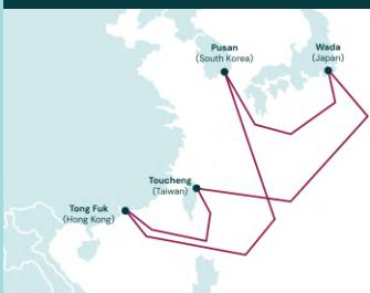
A Resilient loop cable offering protected and unprotected capacity options with connectivity into Taiwan, Hong Kong, Japan & South Korea. The cable is extended to popular interconnect locations enabling seamless connectivity to South-East Asia and US.
